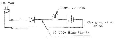
This charger will work somewhat on 9V transistor batteries, but does a good job on Ni-Cads. I have charged one 1.2V Ni-Cad and I have charged eight 5V Ni-Cads in SERIES. It works as is.
