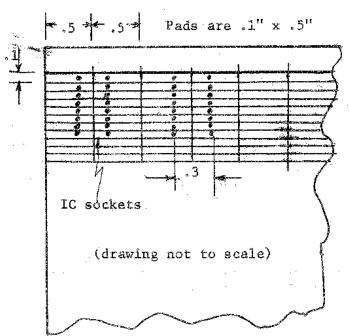
Drill holes for sockets and mount Solder #32 wire to pads, pont to point
