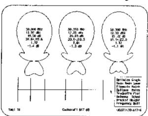
The plots shown above are screen dumps of the main YO screen. The numbers inside each beam pattern are, from top to bottom, frequency, forward gain, front to rear ratio, input impedance, matched standing wave ratio, and figure of merit. The plot on the left of the next page shows overlays the two antenna's beam plots. The graphs on the right plots the gain, F/R, SWR, and impedance verses frequency for the new design.
